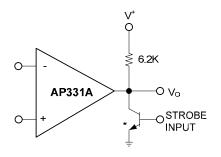
\* OR LOGIC GATE WITHOUT PULL-UP RESISTOR
