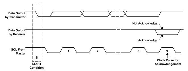
Figure 43. Acknowledge on the I<sup>2</sup>C Bus
