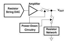
Figure 46. Output Stage During Power Down
