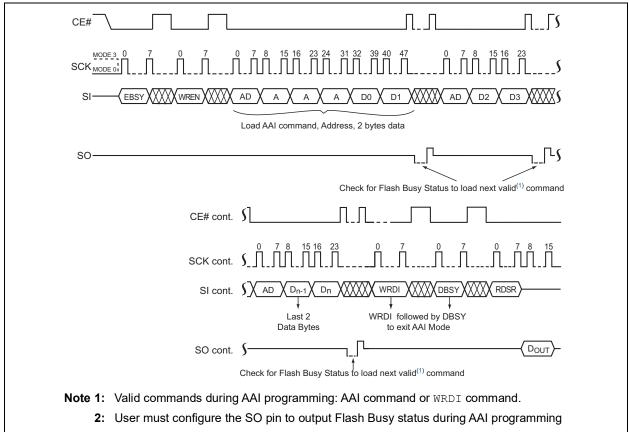
FIGURE 4-9: AUTO ADDRESS INCREMENT (AAI) WORD PROGRAM SEQUENCE WITH SOFTWARE END OF WRITE DETECTION
