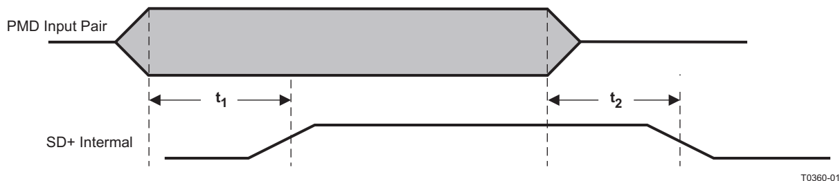
Figure 9-20. 100Base-TX Signal Detect Timing
