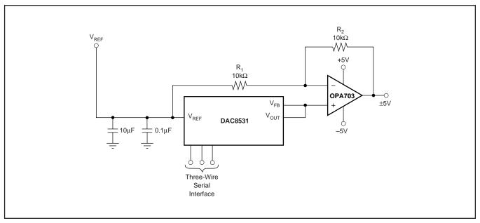
FIGURE 10. Bipolar Operation with the DAC8531.
