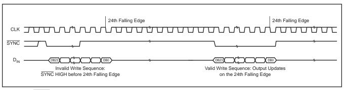
FIGURE 4. SYNC Interrupt Facility.
