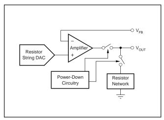
FIGURE 5. Output Stage During Power-Down.
