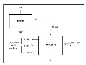
FIGURE 9. REF02 as a Power Supply to the DAC8531.
