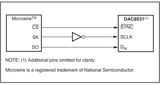
FIGURE 7. DAC8531 to Microwire Interface.
