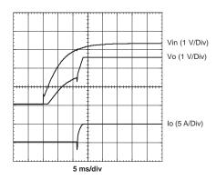
Figure 14. Pre-Bias Startup Waveforms
