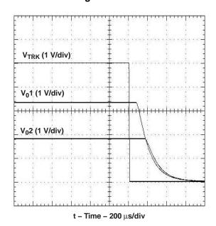
Figure 12. Simultaneous Power Down With Auto-Track Control
