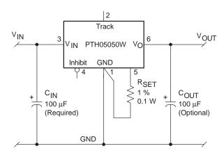
Figure 5. Vo Adjust Resistor Placement
