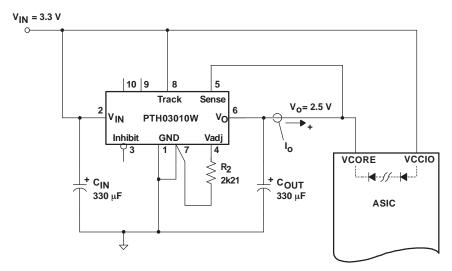
Figure 13. Application Circuit Demonstrating Pre-Bias Startup
