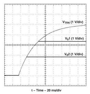
Figure 11. Simultaneous Power Up With Auto-Track Control
