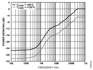
Figure 2. RF Input Power Derating
