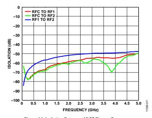
Figure 11. Isolation Between All RF Pins vs. Frequency in All Off State (EN =  $V_{DD}$ )
