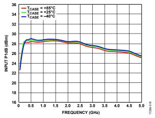
Figure 18. Input P1dB vs. Frequency over Temperature,  $V_{DD} = 3 V$
