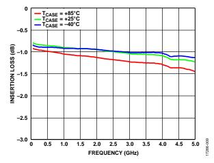
Figure 9. Insertion Loss Between RFC and RF2 vs. Frequency over Temperature
