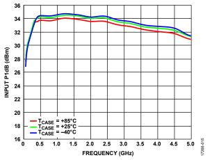
Figure 15. Input 1 dB Power Compression (P1dB) vs. Frequency over Temperature,  $V_{DD} = 5 \text{ V}$
