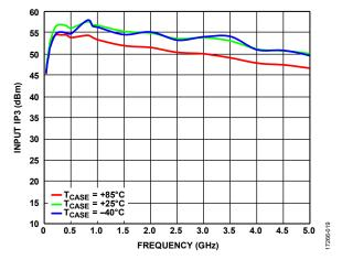
Figure 19. Input IP3 vs. Frequency over Temperature,  $V_{DD} = 3 \text{ V}$
