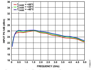
Figure 17. Input P0.1dB vs. Frequency over Temperature,  $V_{DD} = 3 V$
