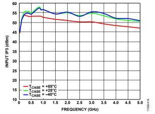
Figure 16. Input IP3 vs. Frequency over Temperature,  $V_{DD} = 5 V$
