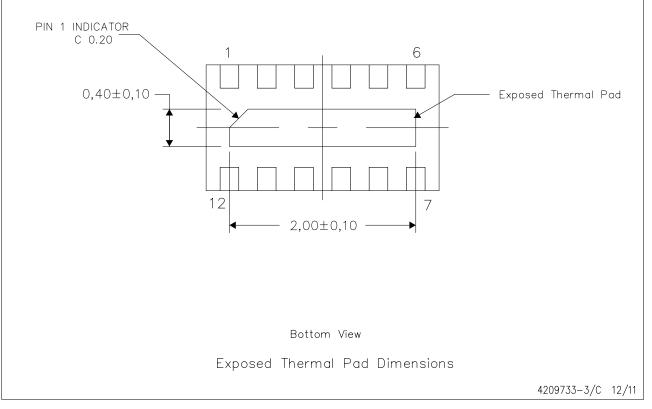
NOTE: All linear dimensions are in millimeters
