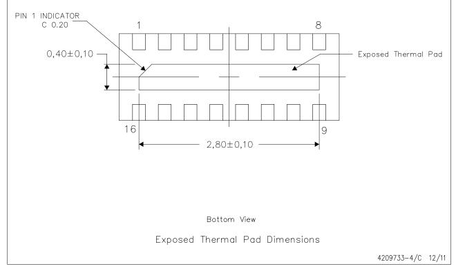
NOTE: All linear dimensions are in millimeters
