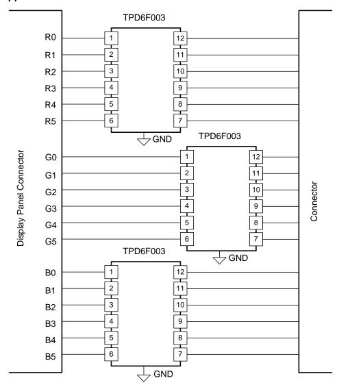
Figure 10. Display Panel Schematic
