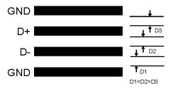
Figure 19. Ideal Diode Trace Layout
