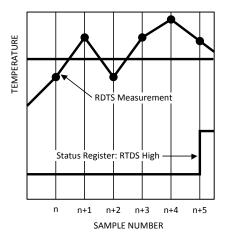
Figure 14. Fault Queue Temperature Response Diagram
