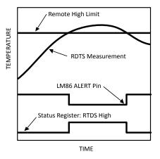
Figure 4. ALERT Comparator Temperature Response Diagram
