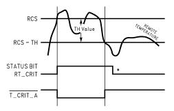
\* Note: Status Register Bits are reset by a read of Status Register.
