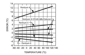
Figure 16. Error Caused by Nonideality Factor
