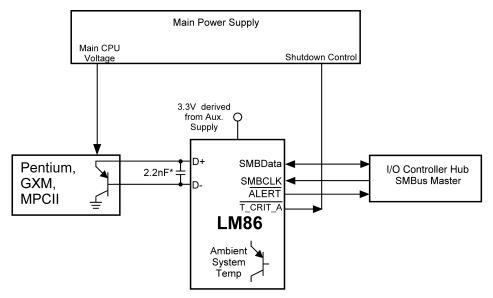
\*Note: 2.2nF Capacitor must be placed as close as possible to D+ and D- pins of the LM86.
