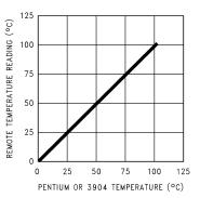
Figure 15. Mobile Pentium III or 3904 Temperature vs LM86 Temperature Reading
