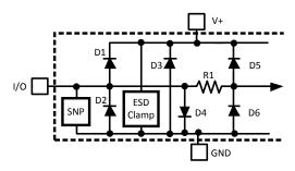
Figure 1. ESD Protection Input Structure
