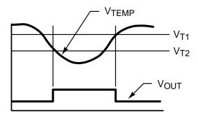
Figure 17. Thermostat Output Waveform
