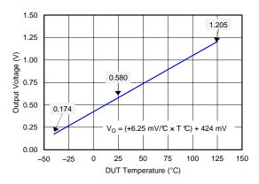
Figure 15. LM60-Q1 Output Transfer Function
