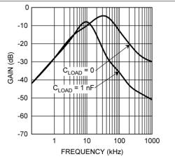
Figure 8. Supply-Noise Gain vs Frequency
