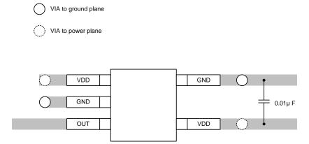
Figure 19. SC70 Package Recommended Layout
