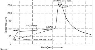
I.Recommend pre-heat temperature of 105°C or less (as measured with a thermocouple attached to the LED pins) prior to immersion in the solder wave with a maximum solder bath temperature of 260°C
