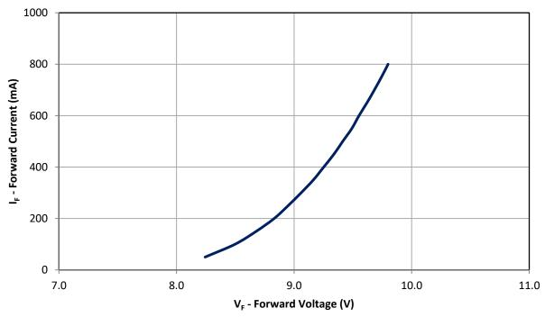
Figure 10: Typical forward current vs. forward voltage<sup>1</sup> @  $T_c = 25^{\circ}C$ .
