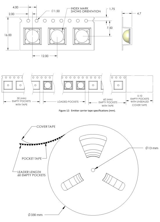
Figure 13: Emitter Reel specifications (mm).
