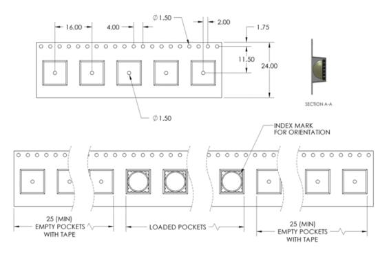
Figure 12: Emitter carrier tape specifications (mm).
