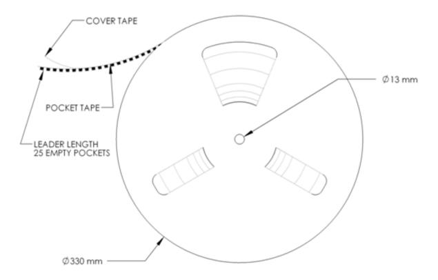
Figure 13: Emitter Reel specifications (mm).
