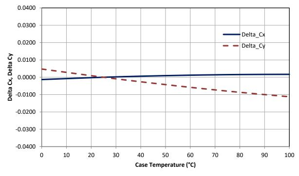
Figure 9: Typical chromaticity coordinate shift vs. Case temperature  $\label{eq:figure} \begin{tabular}{ll} \end{tabular}$
