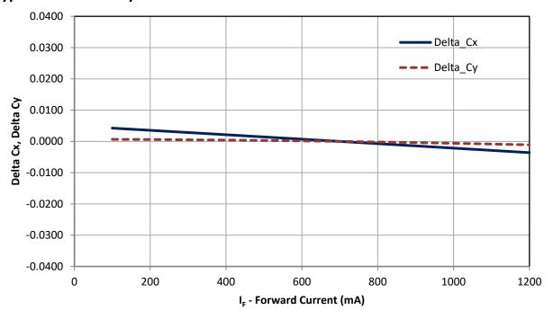
Figure 8: Typical chromaticity coordinate shift vs. forward current
