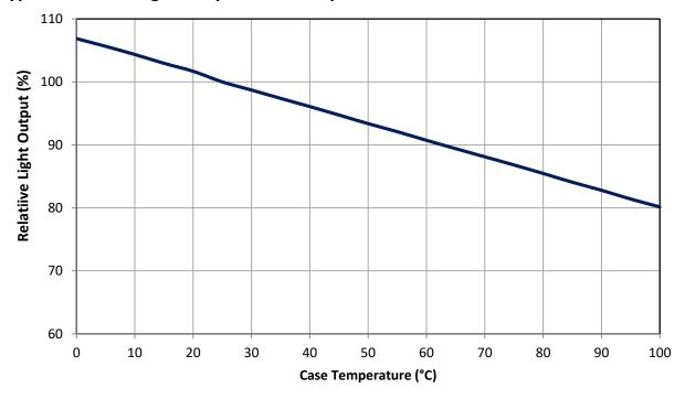
Figure 7: Typical relative light output vs. case temperature.
