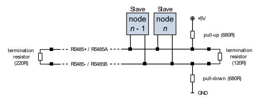
Figure 3.4: Bus lines with resistor (Bias) network on one side, only
