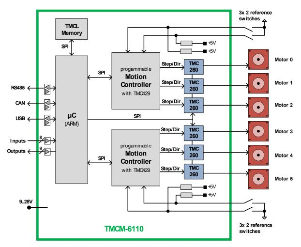
Figure 7.1: TMCM-6110 block diagram
