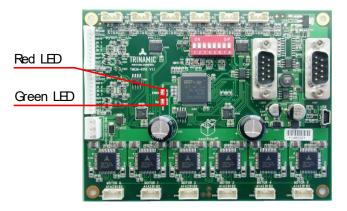
Figure 5.1 On-board LEDs
