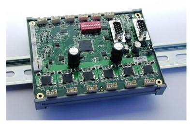
Figure 3.2 DIN rail mounting
