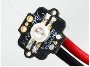
You can use a thinner wire for data, in this case we have a  $^{\sim}22AWG$  data line. It's soldered onto the out pin here
