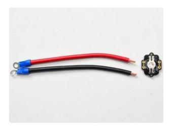
For the power wires, make sure to get nice hefty ones that can handle the current draw. Of course, it matters how long they're going to be, and how many Pixies are in the chain, and how much they will be lit up. 16 AWG is the recommended size.
