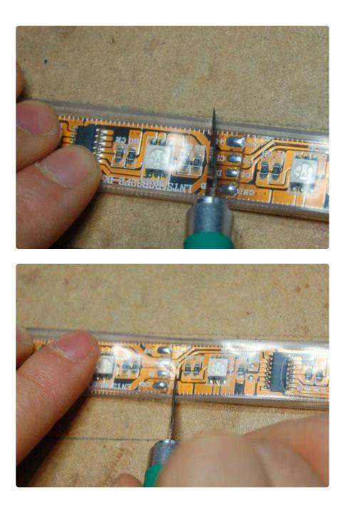
Then slice the rubber coating between the two cuts you made:
