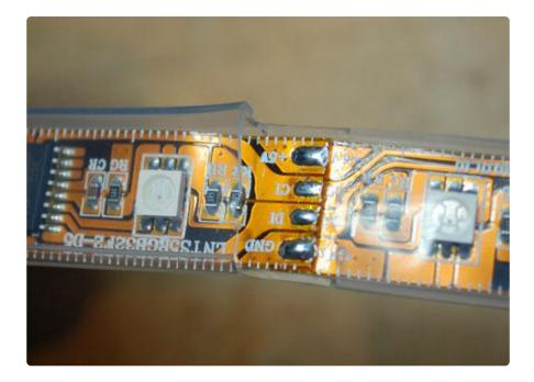
Press the soldering iron against the four joints while pulling the two pieces apart:
