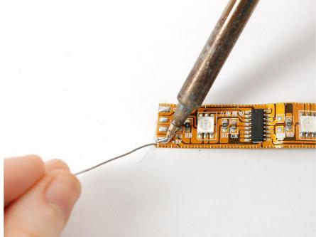
Start by soldering a red wire to the +5V power line:
