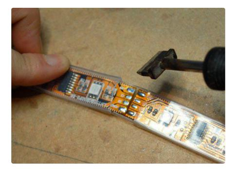
Cut the remaining rubber underneath with scissors:
