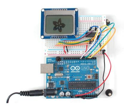
You can control the backlight, its much brighter when you connect the backlight pin to 5V (you don't need a level shifter if you are using a Nokia display from Adafruit). You can control the backlight using an Arduino pin since there is a transistor on the board.
