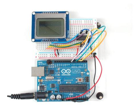
You can save some pins by connecting the CS pin to ground (this means you cant reuse the LCD's pins between screen updates but maybe thats OK. You can also connect the RST pin to the Arduino reset so that it will reset the screen automatically.
