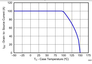
Figure 12. Maximum Drain Current vs Temperature
