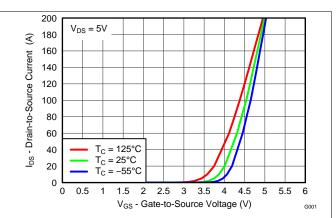
Figure 2. Saturation Characteristics
