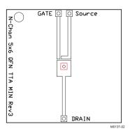
Max  $R_{\theta JA} = 125^{\circ} C/W$  when mounted on a minimum pad area of 2-oz. (0.071-mm thick) Cu.
