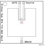
Max  $R_{\theta JA} = 50^{\circ} C/W$  when mounted on 1 inch² (6.45 cm²) of 2-oz. (0.071-mm thick) Cu.
