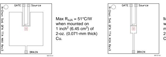
Max  $R_{\theta,JA} = 123^{\circ}C/W$ when mounted on a minimum pad area of 2-oz. (0.071-mm thick) Cu.
