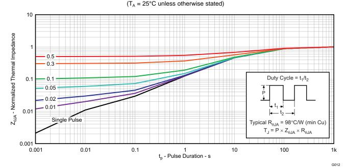
Figure 1. Transient Thermal Impedance
