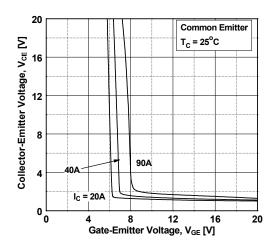
Figure 7. Saturation Voltage vs. V<sub>GE</sub>
