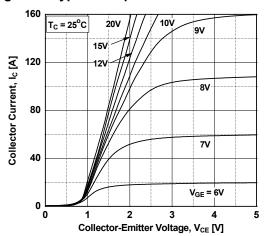
Figure 3. Typical Saturation Voltage Characteristics
