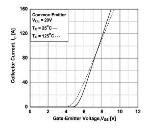
Figure 6. Saturation Voltage vs.  $V_{\text{GE}}$
