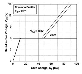
Figure 11. Turn-on Characteristics vs.
