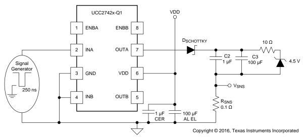
Figure 32. Current Source Capability Test
