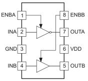
One inverting, one noninverting
