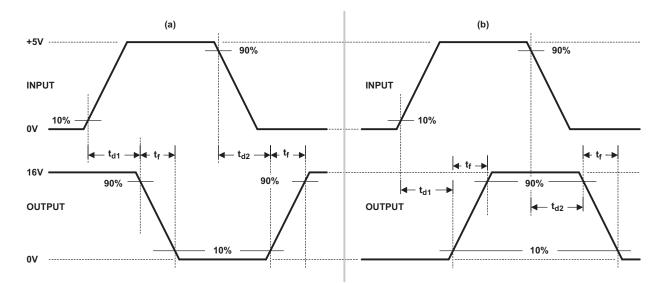
The 10% and 90% thresholds depict the dynamics of the bipolar output devices that dominate the power MOSFET transition through the Miller regions of operation.
