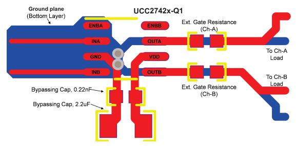
Figure 35. Recommended PCB Layout for UCC2742x-Q1
