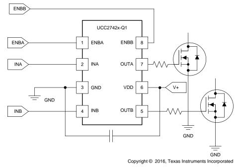
Figure 30. UCC2742x-Q1 Driving Two Independent MOSFETs
