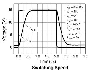
High Load Capacitance  $C_1 = 100nF$
