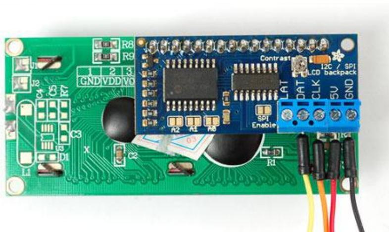
For advanced users, this project can be used for general purpose I/O expansion, the MCP23008 has 8 i/o pins (7 are connected) with optional pullups, the SPI 74HC595 has 7 outputs.
