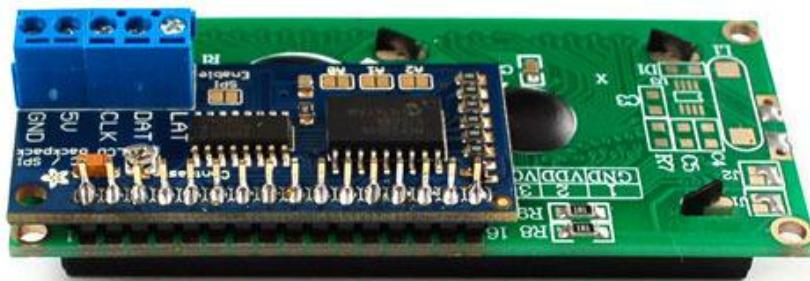
Make sure that as you solder the first pin, the backpack PCB isn't leaning against the LCD, where the terminal blocks could short against some components. You can put some electrical tape or foam tape behind to avoid this if you think it could be an issue.
