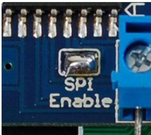
This will switch the backpack over to SPI mode instead of i2c. If you want to go back to i2c, use wick or a solder sucker to remove the jumper
