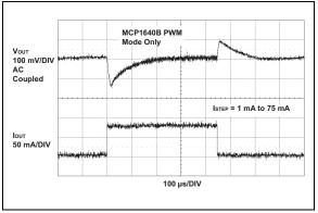
**FIGURE 2-22:** MCP1640B 3.3V V<sub>OUT</sub> Load Transient Waveforms.
