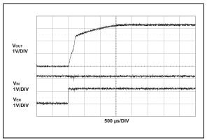
FIGURE 2-19: 3.3V Start-Up After Enable.
