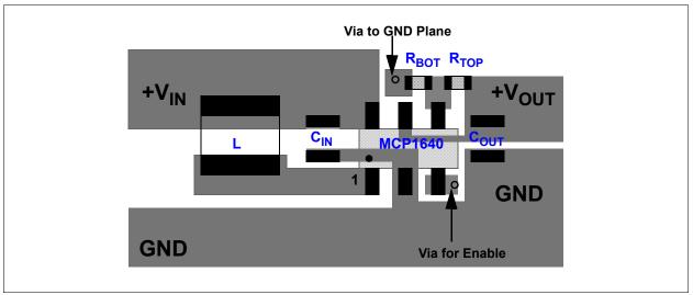
FIGURE 5-1: MCP1640/B/C/D SOT-23-6 Recommended Layout.
