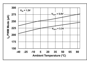
**FIGURE 2-2:**  $V_{OUT} I_Q$  vs. Ambient Temperature in PWM Mode.
