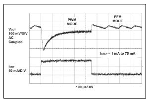
**FIGURE 2-21:** MCP1640 3.3V V<sub>OUT</sub> Load Transient Waveforms.
