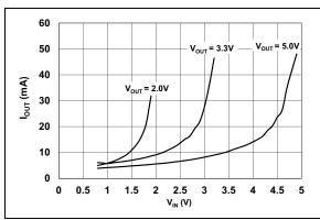
**FIGURE 2-15:** Average of PFM/PWM Threshold Current vs.  $V_{IN}$ .
