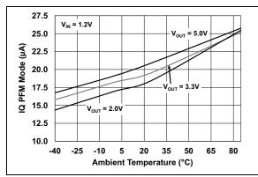
**FIGURE 2-1:**  $V_{OUT}I_Q$  vs. Ambient Temperature in PFM Mode.
