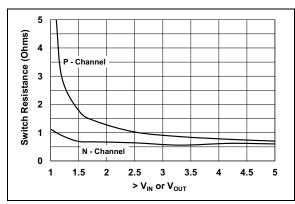
**FIGURE 2-14:** N-Channel and P-Channel  $R_{DSON}$  vs. > of  $V_{IN}$  or  $V_{OUT}$ .
