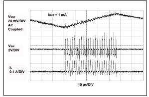
**FIGURE 2-16:** MCP1640 3.3V V<sub>OUT</sub> PFM Mode Waveforms.
