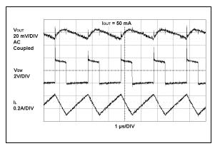
FIGURE 2-18: MCP1640/B High Load Waveforms.
