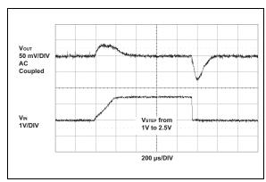
**FIGURE 2-24:** 3.3V V<sub>OUT</sub> Line Transient Waveforms.
