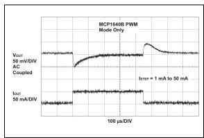
FIGURE 2-23: MCP1640B 2.0V V<sub>OUT</sub> Load Transient Waveforms.
