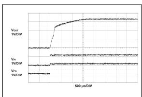
FIGURE 2-20: 3.3V Start-Up when  $V_{IN} = V_{ENABLE}$ .
