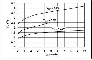
FIGURE 2-12: Threshold vs. I<sub>OUT</sub>.
