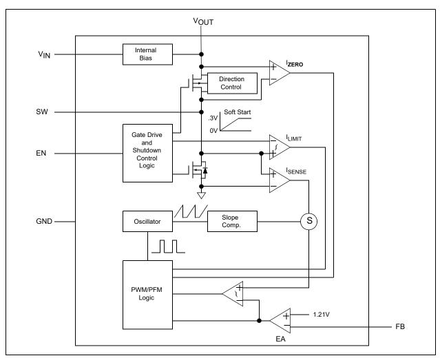
FIGURE 4-1: MCP1640/B/C/D Block Diagram.
