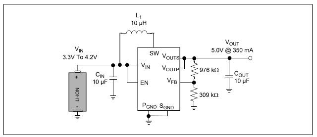
FIGURE 6-2: USB On-The-Go Powered by Li-Ion Battery.
