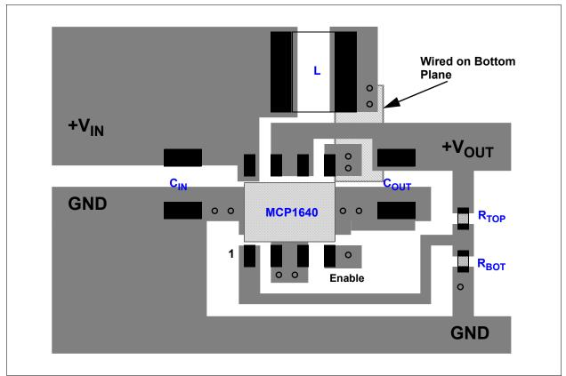
FIGURE 5-2: MCP1640/B/C/D DFN-8 Recommended Layout.
