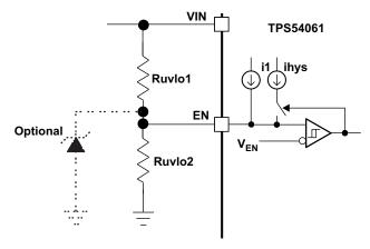
Figure 18. Adjustable Undervoltage Lock-Out
