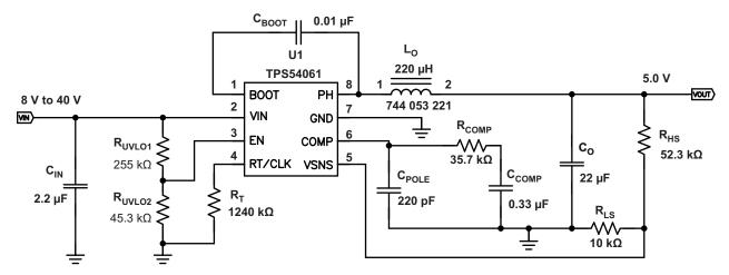
Figure 38. DCM Application Schematic
