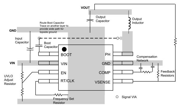
Figure 54. PCB Layout Example
