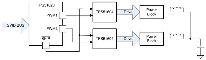
Figure 3-1. Simplified Schematic
