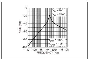
**FIGURE 2-4:** Power Supply Rejection Ratio.
