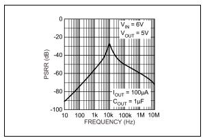
**FIGURE 2-1:** Power Supply Rejection Ratio.
