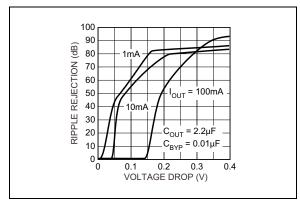
**FIGURE 2-6:** Power Supply Ripple Rejection vs. Voltage Drop.
