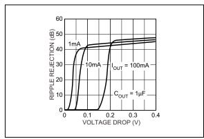
**FIGURE 2-3:** Power Supply Ripple Rejection vs. Voltage Drop.
