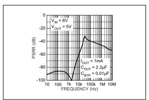
**FIGURE 2-5:** Power Supply Rejection Ratio.
