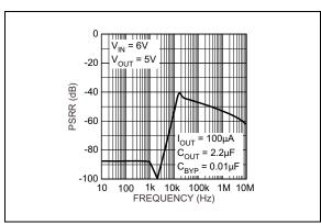
**FIGURE 2-2:** Power Supply Rejection Ratio.
