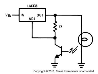
Figure 31. 5-V Logic Regulator With Electronic Shutdown\*\*
