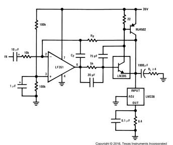
$A_V = 1$ ,  $R_F = 10k$ ,  $C_F = 100$  pF  $A_V = 10$ ,  $R_F = 100k$ ,  $C_F = 10$  pF Bandwidth  $\ge 100$  kHz Distortion  $\le 0.1\%$
