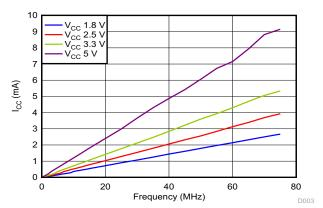
Figure 9-2. I<sub>CC</sub> vs Frequency
