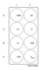
Figure 5-2. YZP Package 8-Pin DSBGA Bottom View
