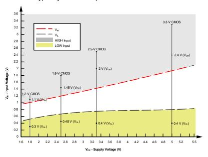
Figure 9-3. LVxT Input Voltage Levels
