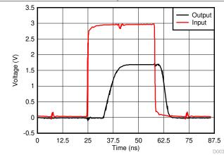
Figure 7-3. Switching Characteristics at 15 MHz Excellent Signal Integrity
