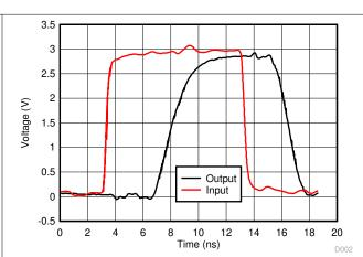
Figure 7-2. Switching Characteristics at 50 MHz Excellent Signal Integrity
