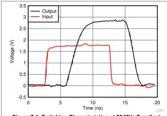
Figure 7-1. Switching Characteristics at 50 MHz Excellent Signal Integrity
