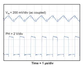
Figure 29. INPUT VOLTAGE RIPPLE,  $I_{OUT} = 3 A$
