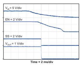
Figure 27. SHUT DOWN RELATIVE TO VIN
