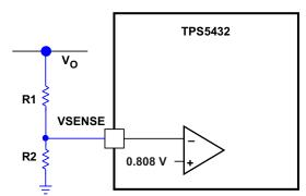
Figure 17. Voltage Divider Circuit
