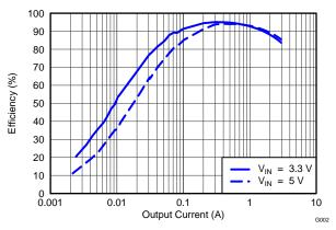
Figure 22. EFFICIENCY vs LOAD CURRENT
