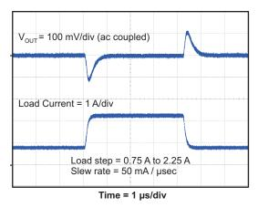
Figure 23. TRANSIENT RESPONSE, 1.5 A STEP
