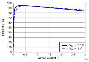
Figure 21. EFFICIENCY vs LOAD CURRENT
