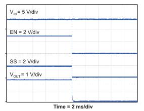
Figure 28. SHUT DOWN RELATIVE TO EN
