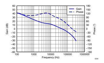
Figure 24. CLOSED LOOP RESPONSE,  $V_{IN}$  = 5 V,  $I_{OUT}$  = 1.5 A
