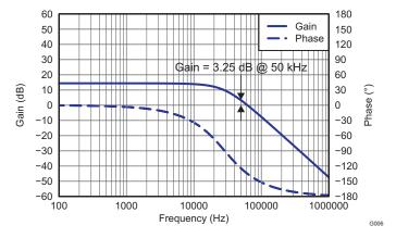
Figure 20. Power Stage Gain and Phase Characteristics
