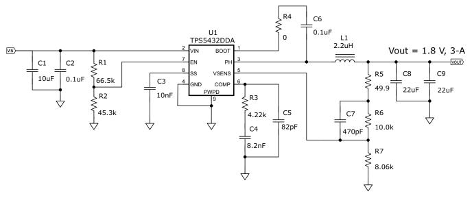
Figure 19. 1.8 V Output Power Supply Design with Adjustable UVLO
