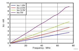
Figure 9-2. I<sub>CC</sub> vs Frequency
