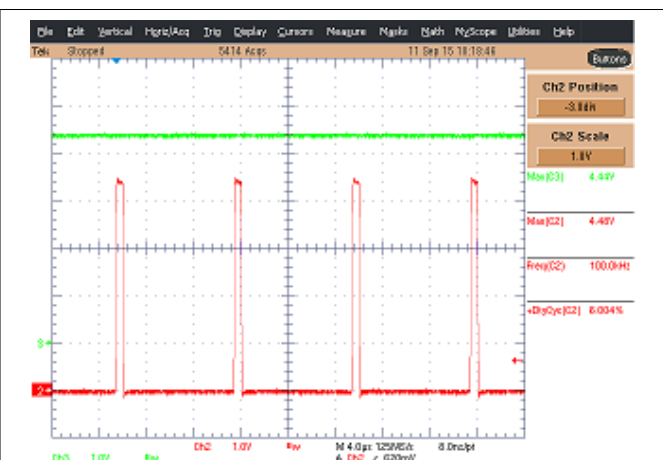
Figure 8-9. Supply Voltage 5 V Peak Signal 4.5 V
