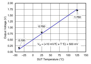
Figure 15. Output Transfer Function
