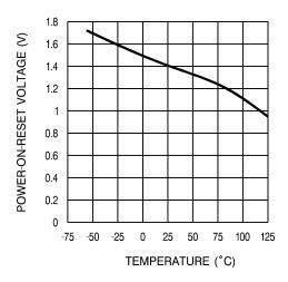
Figure 6. Average Power on Reset Voltage vs Temperature
