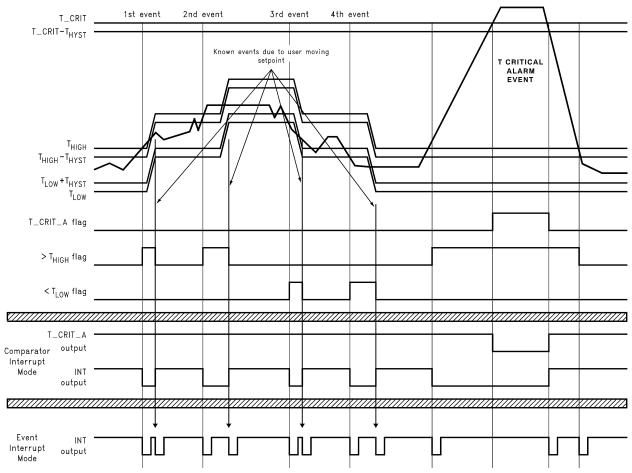
**Note:** Event Interrupt mode is drawn as if the user is reading the part. If the user doesn't read, the outputs would go low and stay that way until the LM92 is read.
