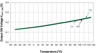
Output ON Voltage vs Temperature
