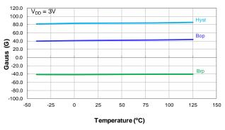
Switch Points Bop and Brp vs Temperature
