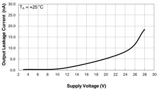
Output Leakage Current vs Supply Voltage
