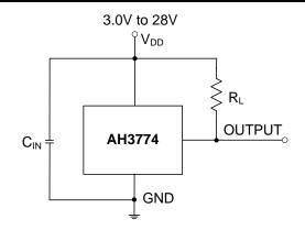
Note: 4. C<sub>IN</sub> is for power stabilization and to strengthen the noise immunity, the recommended capacitance is 10nF ~ 100nF. RL is the pull-up resistor.
