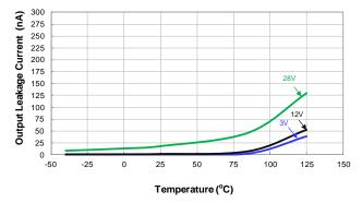
Output Leakage Current vs Temperature
