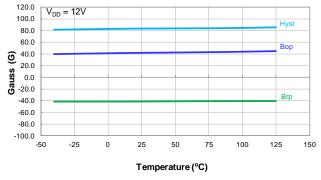
Switch Points Bop and Brp vs Temperature
