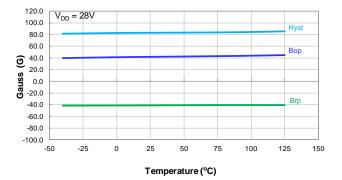
Switch Points Bop and Brp vs Temperature
