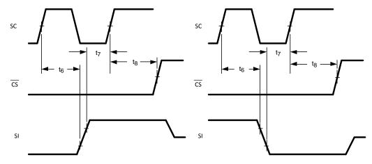
Figure 3. Data Input Timing Diagram
