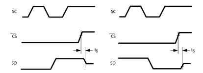
Figure 2. TRI-STATE Data Output Timing Diagram
