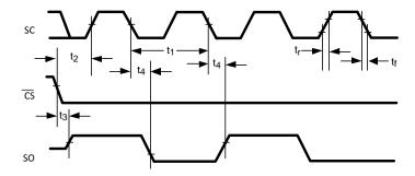
Figure 1. Data Output Timing Diagram
