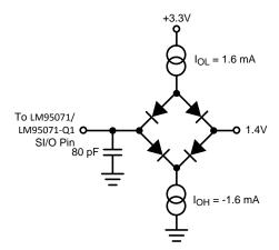
Figure 9. TRI-STATE Test Circuit
