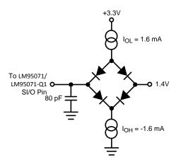
Figure 9. TRI-STATE Test Circuit
