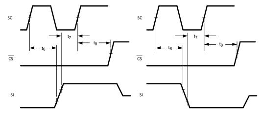
Figure 3. Data Input Timing Diagram
