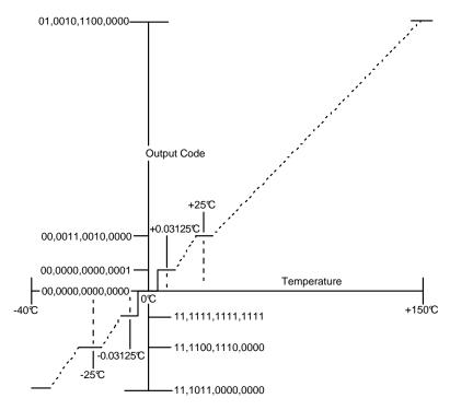
Figure 8. Temperature-to-Digital Transfer Function (Non-Linear Scale for Clarity)
