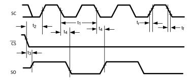
Figure 1. Data Output Timing Diagram
