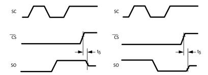
Figure 2. TRI-STATE Data Output Timing Diagram
