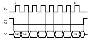
Figure 10. Reading Continuous Conversion - Single Eight-Bit Frame
