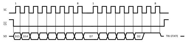
Figure 11. Reading Continuous Conversion - Two Eight-Bit Frames
