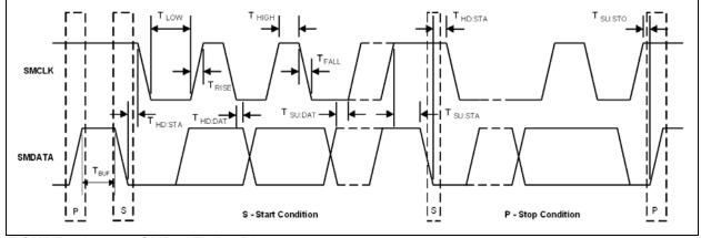
FIGURE 4-1: SMBus Timing Diagram.
