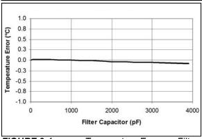
**FIGURE 2-1:** Temperature Error vs. Filter Capacitor (2N3904,  $T_A = 27^{\circ}C$ ,  $V_{DD} = 3.3V$ ).
