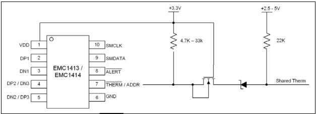
FIGURE 4-2: Isolating the THERM Pin.
