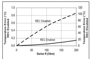
**FIGURE 2-5:** Temperature Error vs. Series Resistance.
