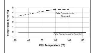
**FIGURE 2-4:** Temperature Error vs. CPU Temperature; Typical 65 nm CPU from Major Vendor ( $T_A = 27^{\circ}$ C,  $V_{DD} = 3.3$ V, BETA = 011,  $C_{FILTER} = 470 \text{ pF}$ ).
