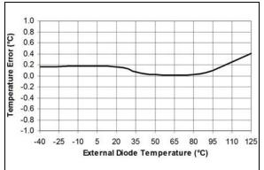
**FIGURE 2-2:** Temperature Error vs. External Diode Temperature (2N3904,  $T_A = 42.5^{\circ}$ C,  $V_{DD} = 3.3V$ ).
