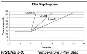
FIGURE 5-3: Temperature Filter Step Response.
