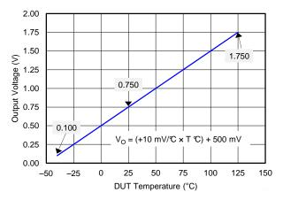
Figure 15. Plot of Output Transfer Function
