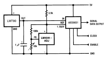
Figure 16. Centigrade Thermostat / Fan Controller
