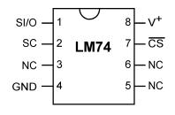
Figure 2. SOIC – Top View See Package Number D
