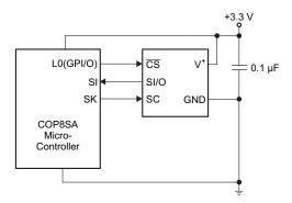
Figure 4. COP Microcontroller Interface
