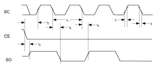
Figure 5. Data Output Timing Diagram
