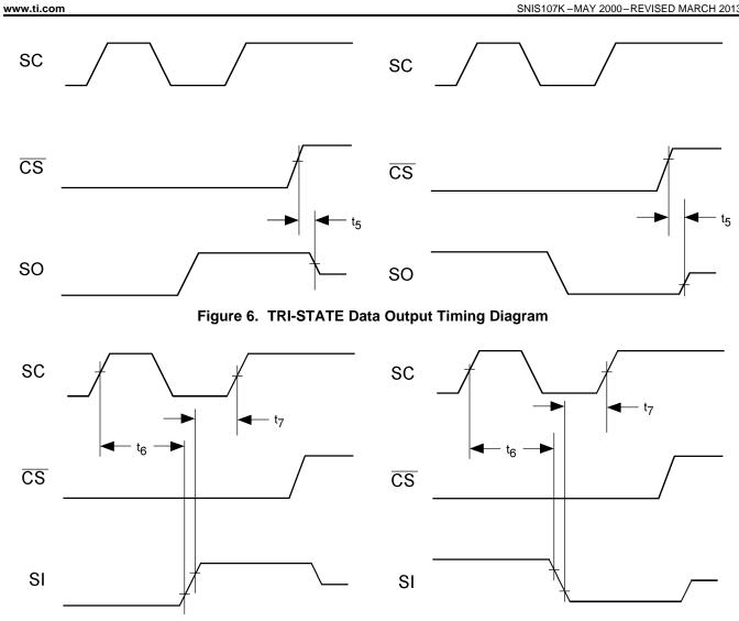
Figure 7. Data Input Timing Diagram
