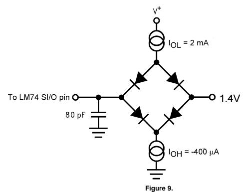
**TRI-STATE Test Circuit**
