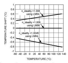
Figure 17. Errors Induced when Temperature Sensor is Not Calibrated to Typical Non-Ideality
