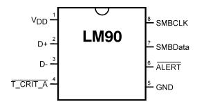
Figure 1. 8-Lead VSSOP - TOP VIEW See DGK Package
