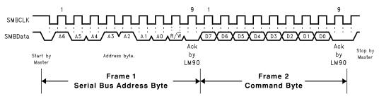
Figure 9. (b) Serial Bus Write to the Internal Command Register
