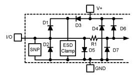
Figure 2. ESD Protection Input Structure
