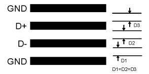
Figure 19. Ideal Diode Trace Layout
