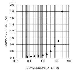
Figure 3. Conversion Rate Effect on Power Supply Current
