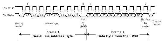
Figure 10. (c) Serial Bus Read from a Register with the Internal Command Register preset to desired value
