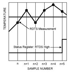
Figure 14. Fault Queue Temperature Response Diagram
