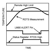
Figure 4. ALERT Comparator Temperature Response Diagram
