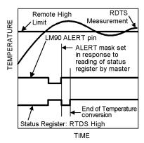
Figure 5. ALERT Output as an Interrupt Temperature Response Diagram
