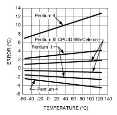
Figure 16. Error Caused by Non-Ideality Factor
