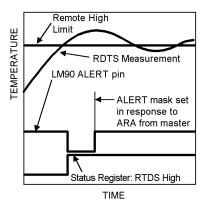
Figure 6. ALERT Output as an SMBus ALERT Temperature Response Diagram
