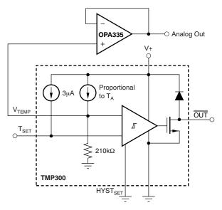
Figure 9. Buffering the Analog Output Signal
