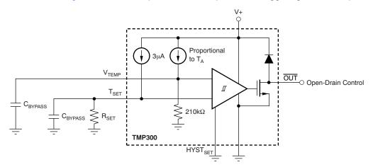
Figure 14. Bypass Capacitors Prevent Early Comparator Toggling Due to Circuit Board Noise
