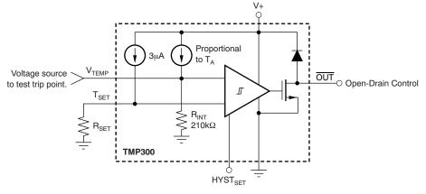
Figure 8. Applying Voltage to Trip Digital Output
