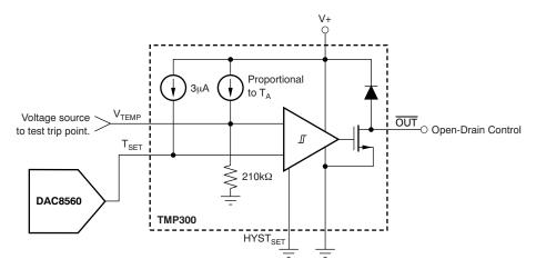
Figure 11. DAC Generates the Voltage-Driving T<sub>SET</sub> Pin
