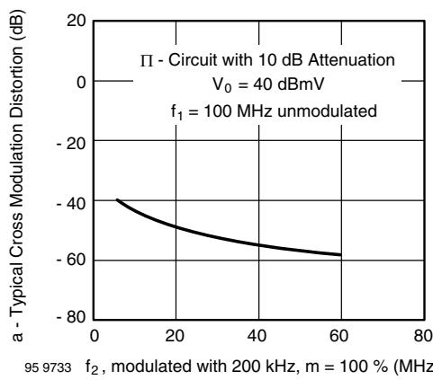
Fig. 3 - Typ. Cross Modulation Distortion vs. Frequency  $f_2$
