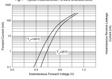
Fig. 1 - Typical Instantaneous Forward Characteristics
