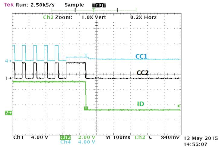
Figure 13. Application Curve for DRP in I<sup>2</sup>C Mode
