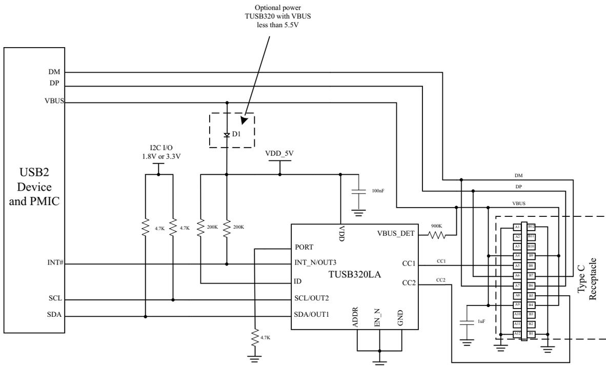
Figure 20. UFP in I<sup>2</sup>C Mode Schematic
