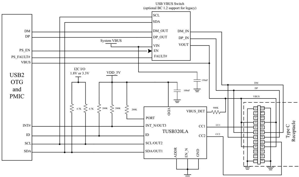
Figure 16. DFP in I<sup>2</sup>C Mode Schematic
