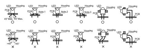
○ " Correct mounting method " x " Incorrect mounting method
