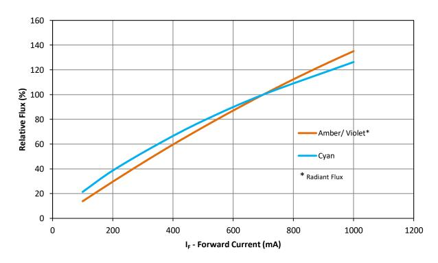
Figure 7b: Typical relative luminous (radiant for Violet) flux vs. forward current @  $T_C = 25^{\circ}C - A$ , C, V
