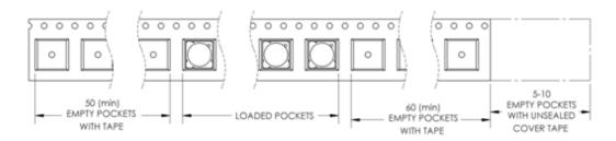
Figure 12: Emitter carrier tape specifications (mm).
