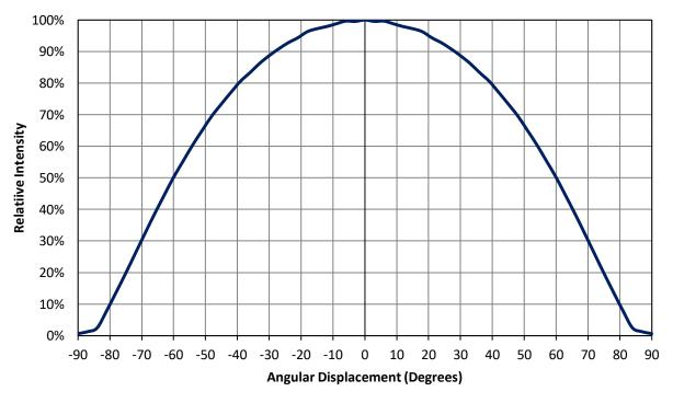
Figure 4: Typical representative spatial radiation pattern – all dies on
