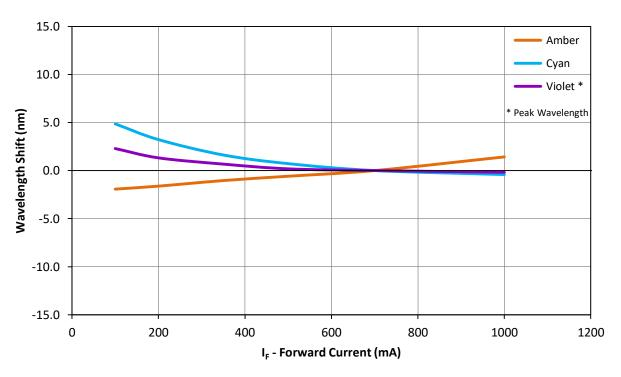
Figure 9b: Typical dominant (peak for Violet) wavelength shift vs. forward current @  $T_c = 25^{\circ}C - A$ , C, V
