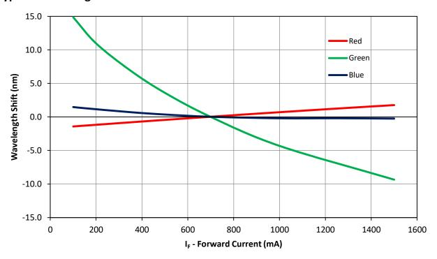
Figure 9a: Typical dominant wavelength shift vs. forward current @  $T_C$  = 25°C – R, G, B
