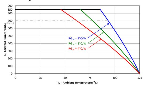
Figure 11: Maximum forward current vs. ambient temperature
