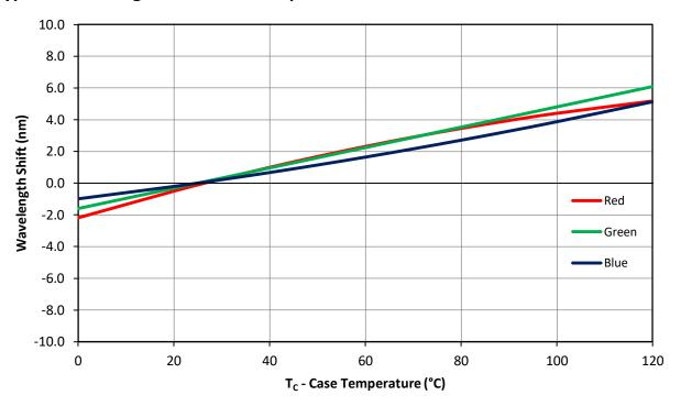
Figure 10a: Typical dominant wavelength shift vs. case temperature - R, G, B
