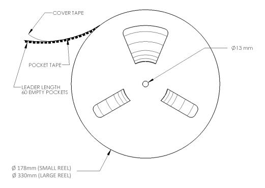
Figure 13: Emitter reel specifications (mm).
