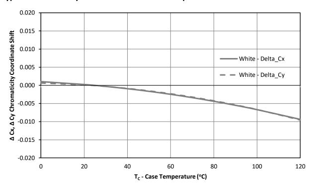
Figure 10c: Typical chromaticity coordinate shift vs. case temperature - White
