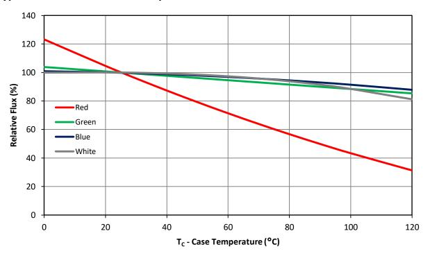
Figure 8a: Typical relative luminous flux vs. case temperature – R, G, B, W
