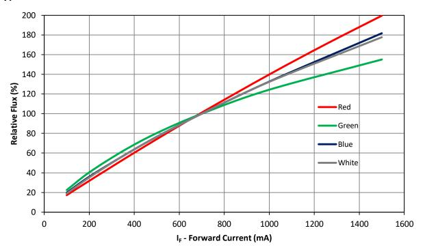
Figure 7a: Typical relative luminous (radiant for Violet) flux vs. forward current @  $T_C = 25^{\circ}C - R$ , G, B, W
