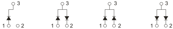
CDBT-40-G Marking Code: 43 CDBT-40S-G Marking Code: 44 CDBT-40C-G Marking Code: 45 CDBT-40A-G Marking Code: 46
